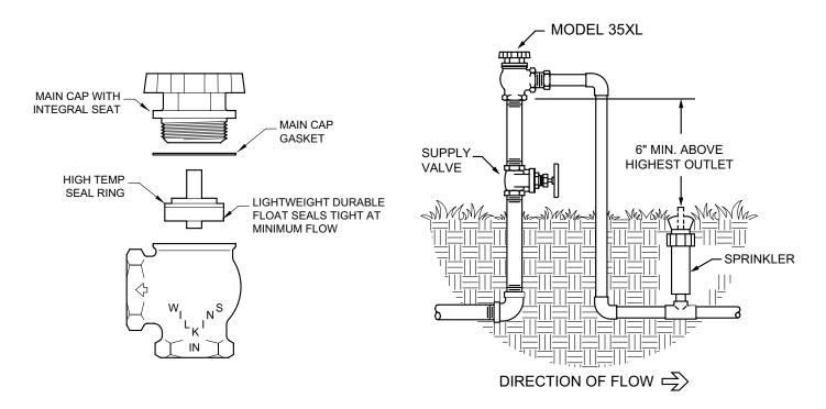
**CAUTION**: This atmospheric vacuum breaker shall not be subjected to continuous pressure for more than twelve (12) hours. The device shall be installed in accordance with the requirements of the local plumbing code. The device shall not be installed where the venting of water from the device during its normal functioning causes damage. The device shall be installed downstream of the last valve, therefore never place a shut off or check valve downstream of AVB's.
