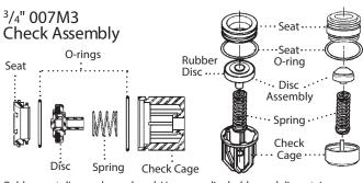
Rubber seat disc can be replaced. However, disc holder and disc retainer are perma water contains less than 0.25% of lead by weight. nently bonded to prevent failure.
